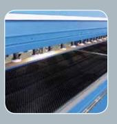
Rectangle holders with synthetic cups to cut narrow strips without being deformed \*NSC system required
