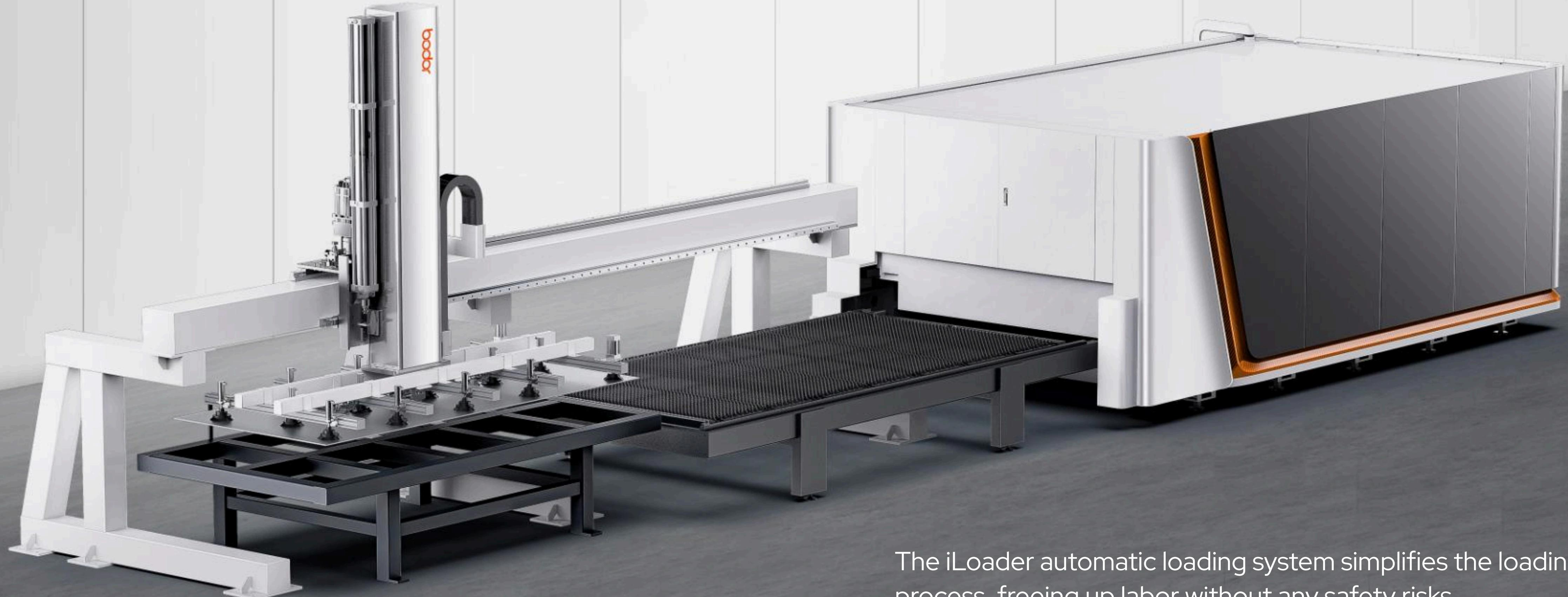
The iLoader automatic loading system simplifies the loading process, freeing up labor without any safety risks.
