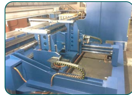
6-axis back gauge, X1-X2-R1-R2-Z1-Z2 (optional)
