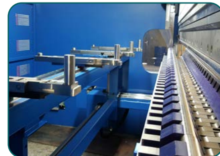
Special made finger stop for thick material (optional)
